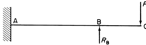
FIGURE 5.11 Analysis of a Propped Cantilever by the Method of Complementary Energy
